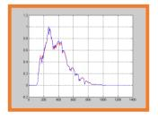
Optical Spectrometry: detects smoke from fires up to 15km away through comparative analysis of sunlight spectra
